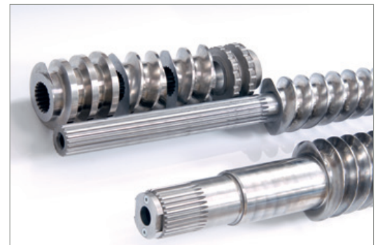
Screw segments: intake, mixing elements, discharge
